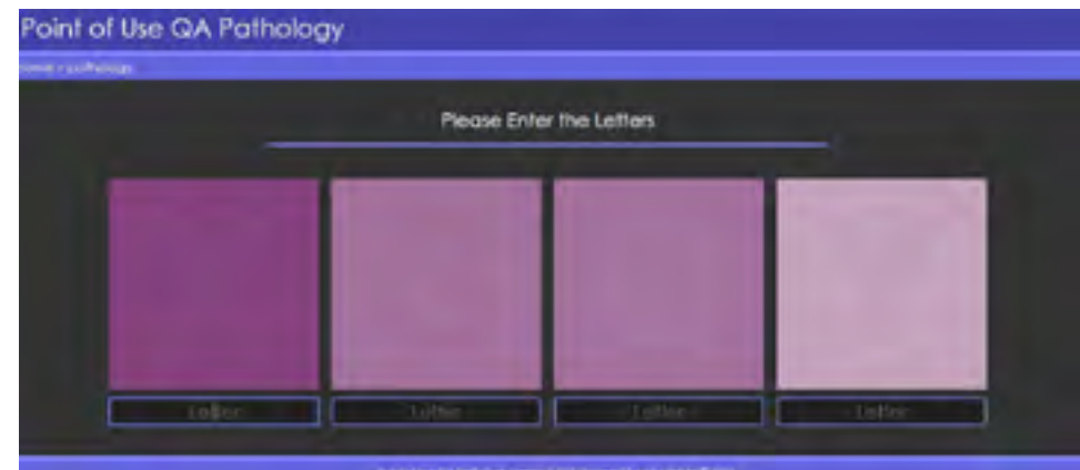
The Point of Use Quality Assurance tool. The user is challenged to identify four letters, which change in each instance of use. In this example, XGQY should be visible on the workstation. Access the tool via https://www.virtualpathology.leeds.ac.uk/research/systems/pouqa/pathology
